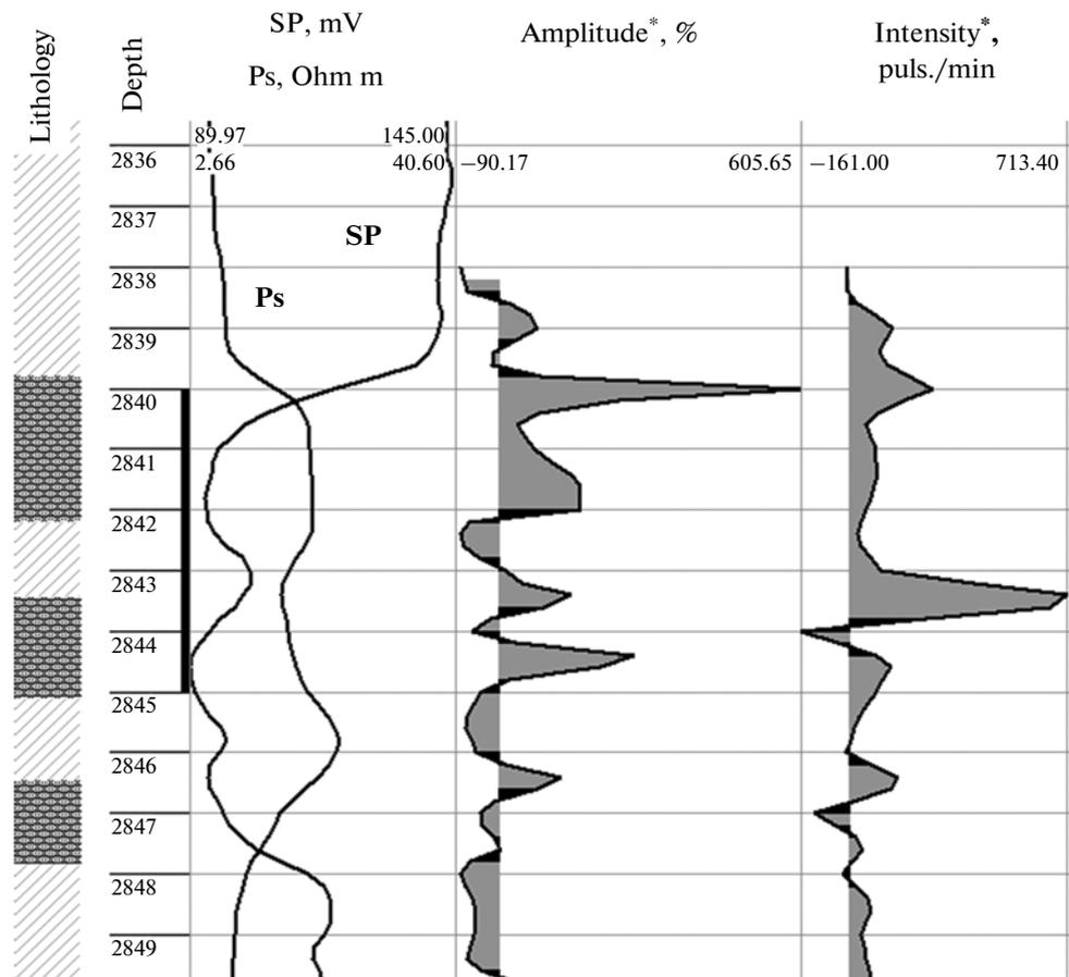
Fig. 3. Diagrams showing results of standard geophysical well logging and seismoacoustic emission measurements.
