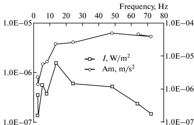
Fig. 7. Fragment of frequency dependence for energy flux density and amplitude of SAE field in the low-frequency part of spectrum.
