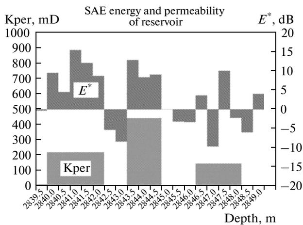
Fig. 4. Comparison of SAE-induced energy and reservoir permeability.
