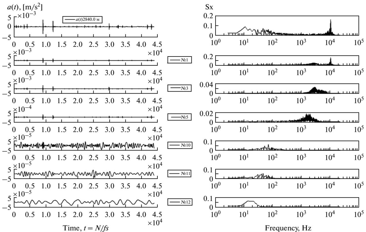
Fig. 5. Example of SAE signal (2-s fragment) decomposition into empirical modes and determination of dominant frequencies.
