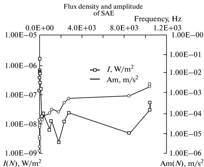
Fig. 6. Frequency dependence for energy flux density and amplitude of SAE field.
